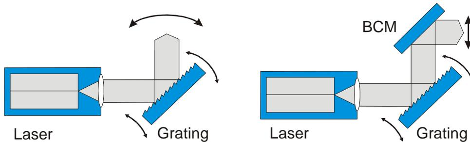
Figure 18: Principle of the beam steering in a Littrow extended cavity diode laser.
