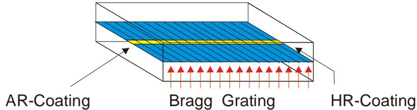
Figure 3: Schematic drawing of a DFB laser diode.
