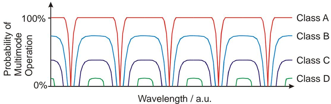
Figure 19: The different classes of antireflection coatings of the laser diode facet.
