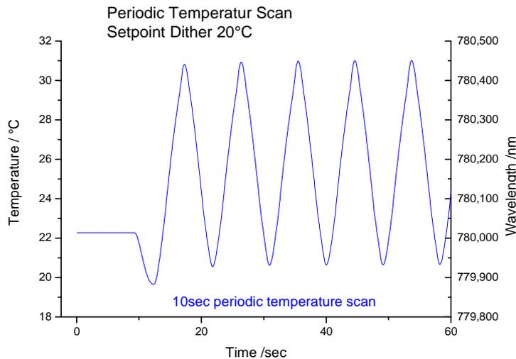
Figure 6: The graphic shows the rapid temperature tuning of a 780nm DFB laser with a low thermal load package. The total temperature change of 10°C results into a wavelength scan of more than 0.4nm. The tuning speed is limited by the thermal capacity of the TO3 or the Butterfly laser package.
