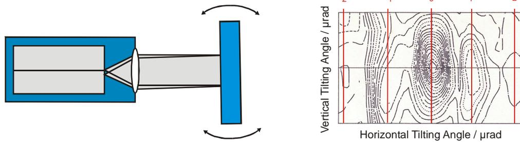
Figure 16: Physical basis of a diode laser with an extended cavity. The left hand side shows one of the possible beam path within an extended optical cavity. The right hand side shows the light intensity of the laser system as a function of the tilting angle of the external cavity mirror as a contour plot. The center of the plot corresponds to the best cavity alignment. The indicated lines show local maxima of the laser intensity for different angles of the external cavity mirror [4].
