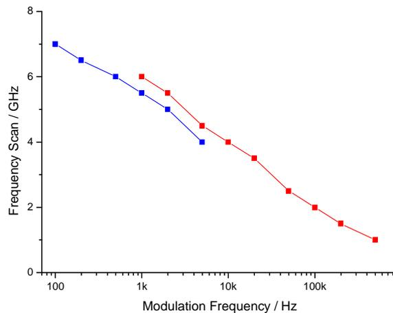
Figure 8: The blue trace shows the modulation response via the P500 modulation input. The red trace shows the modulation response via the BT7 bias tee.
