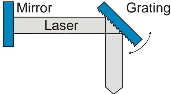
Figure 13: Schematic setup of a tunable laser system with grating feedback.
