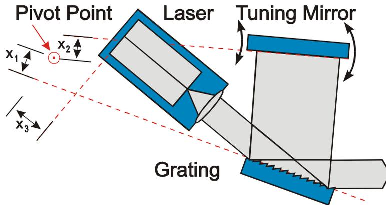
Figure 23: Schematic drawing of an external cavity diode laser system in Littman/Metcalf configuration.
