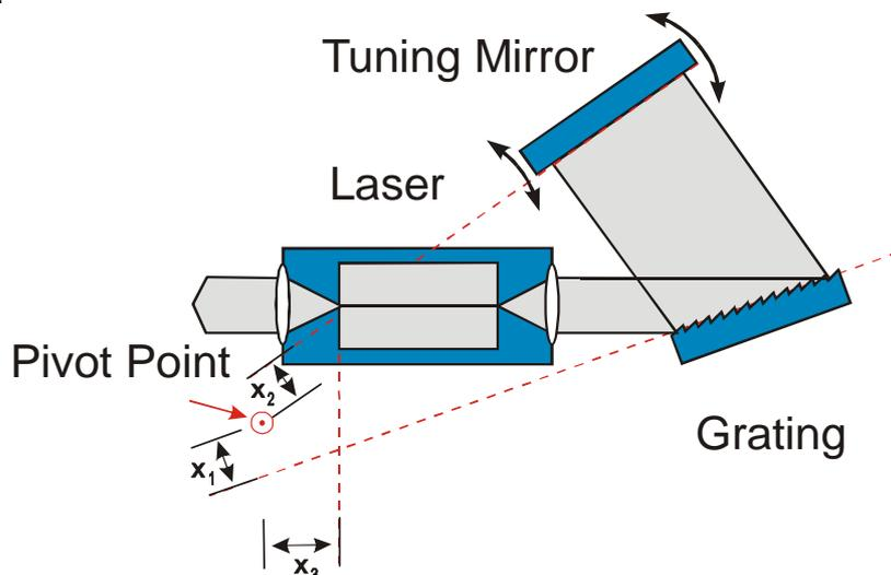
Figure 25: Schematic drawing of an external cavity diode laser system in Littman/Metcalf configuration according to Sacher Lasertechnik.
