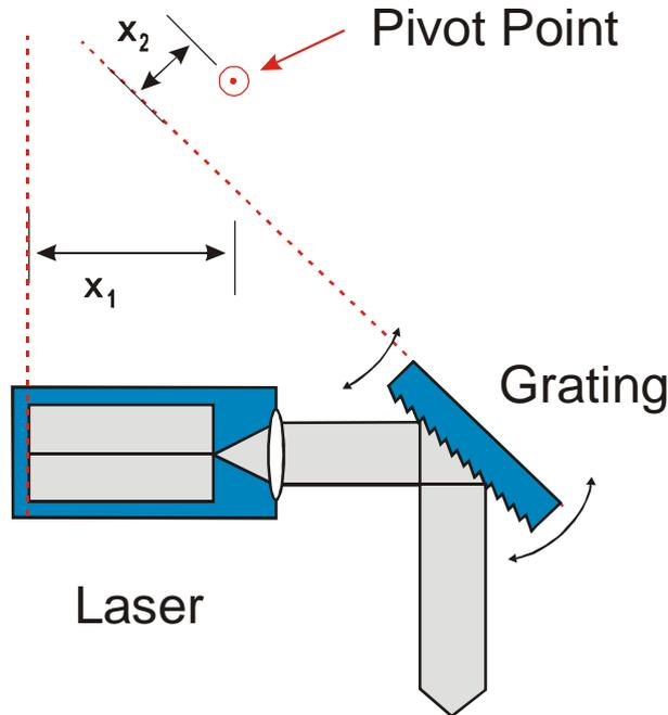
Figure 21: Schematic drawing of an external cavity diode laser system in Littrow configuration.
