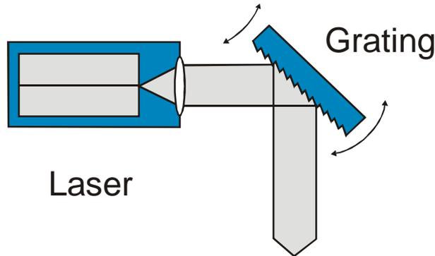
Figure 15: Schematic drawing of an extended cavity diode laser system in Littrow configuration.
