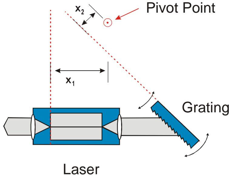
Figure 22: Schematic drawing of an external cavity diode laser system in Littrow configuration according to Sacher Lasertechnik.
