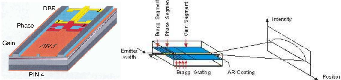
Figure 11. Schematic drawings of the microscopic structure of DBR laser. The left hand side shows the different segments of the DBR laser. The right hand side shows a schematic drawing under a more functional point of view.
