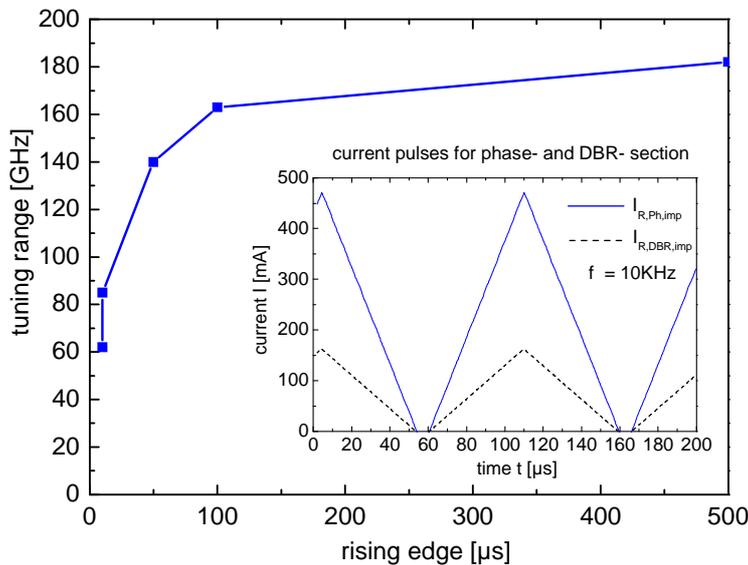
Figure 12. Modulation performance of a DBR laser. The main curve shows the tuning range with different modulation frequencies. The inset describes the ration of DBR and Phase current.
