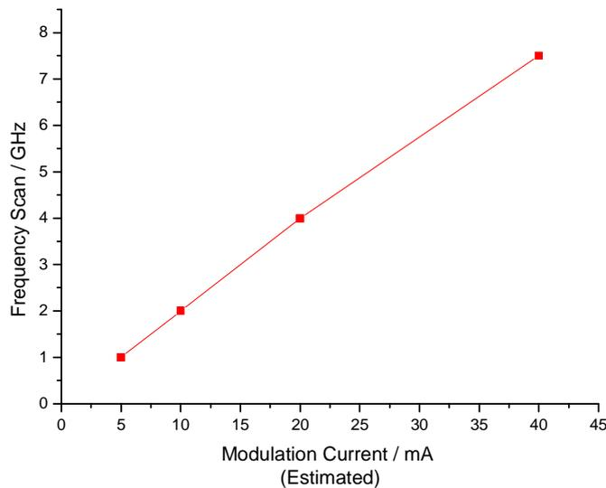
Figure 10. The curve shows an almost linear change of the frequency scan as a function of the modulation amplitude. The tested values range from 5 mA pp to 40 mA pp.
