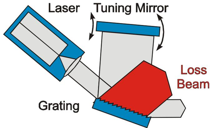
Figure 24: Explanation of the loss beam of the common Littman/Metcalf configuration.
