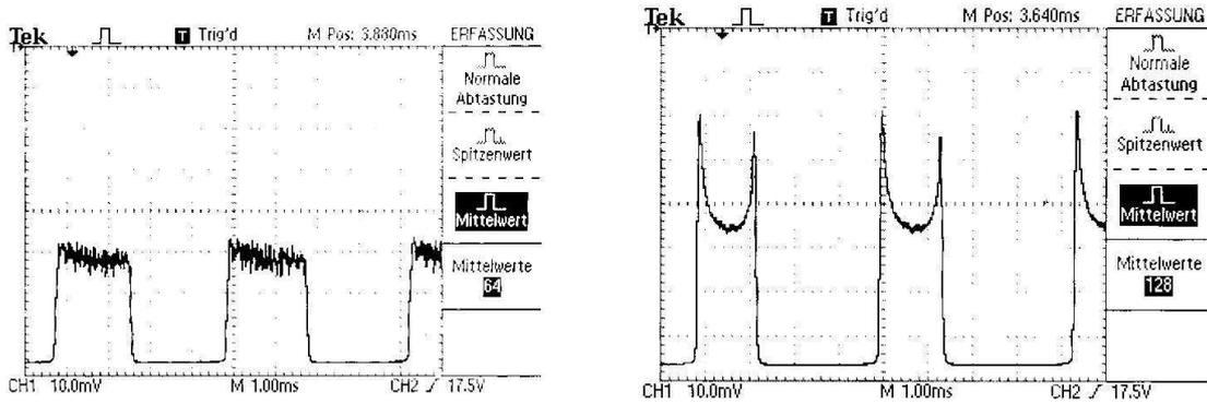
Figure 9. The Fabry Perot spectrum at left hand side shows a modulation response below 10 kHz. The Fabry Perot spectrum at the right hand side shows a modulation response above 100 kHz.
