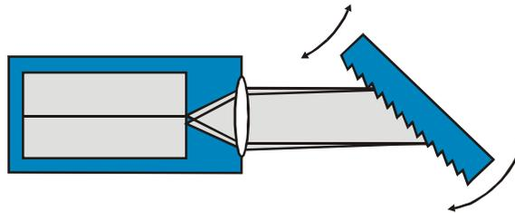
Figure 17: Physical basis of a diode laser with an extended grating cavity. The graph shows one of the possible beam path within the extended optical cavity.
