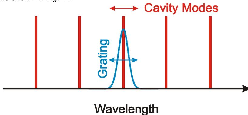
Figure 14: The angle of the diffraction grating and the length of the cavity are changed synchronously to achieve a mode-hop free wavelength tuning.
