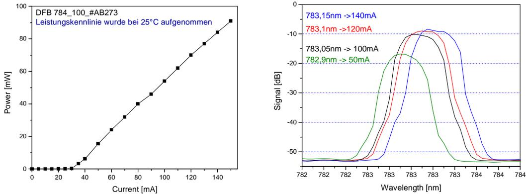
Figure 7: The graph at the left hand side shows the PI curve of the DFB laser. The right hand side graph shows the achieved wavelength tuning. There is only one mode-hop of typically 30GHz right above the laser threshold. Beside this mode-hop, the total injection current tuning is mode-hop-free.
