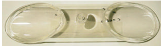
Top and side view of the iodine cell I-100-11 tested for Sacher Lasertechnik
