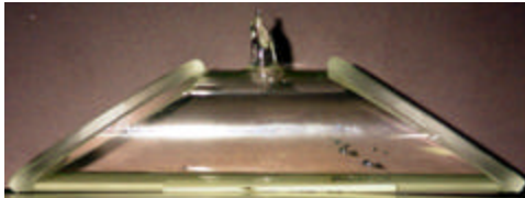
Top and side view of the iodine cell I-100-11 tested for Sacher Lasertechnik
